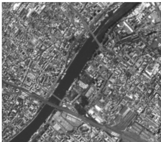
SPOT 5 launched in May 2002 features imaging sensors with 2.5m resolution. This image is of Paris, France.
