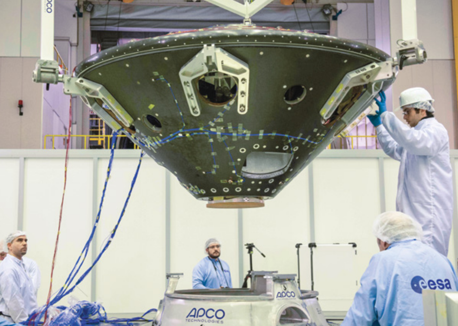
↑ ExoMars Entry, descent, and landing Demonstrator Module being prepared for vibration tests at ESTEC in March 2013
