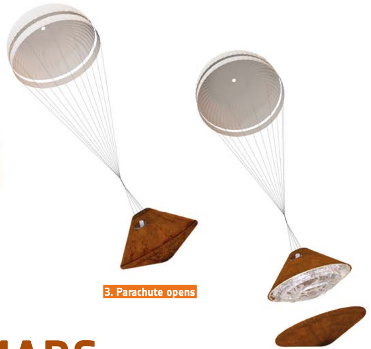
4. Front shield separates, radar turns on
