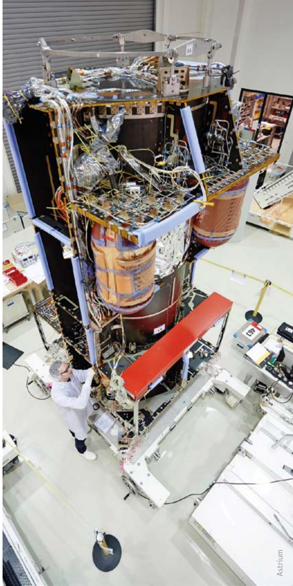
The TGO core module, consisting of the structure and the thermal control and propulsion systems
