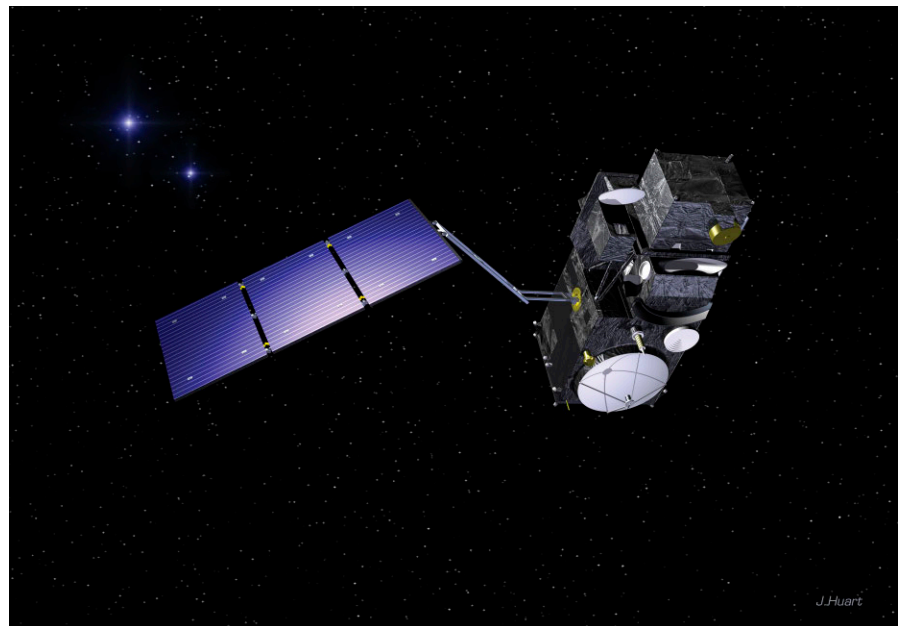
Figure 7. This figure is an artist's rendition of the Sentinel-3 satellite. The SRAL antenna is the larger circular structure on the bottom of the spacecraft. Sentinel-3A will be launched into a Sun-synchronous orbit at 10:00 Local Sidereal Time. Image credit: ESA
