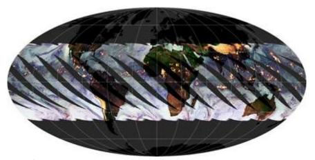
TRMM's low orbital inclination—just 35° from the equator—allows its instruments to concentrate on the tropics. This image shows one half of the observations TRMM makes in a single day. (NASA image courtesy TRMM Project.)
