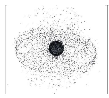
Orbiting objects are concentrated in low Earth orbit (nearly obscuring the Earth's surface in this illustration) and geostationary orbit (revealed by the ring of satellites along the outer edges). (NASA illustration courtesy Orbital Debris Program Office.)
