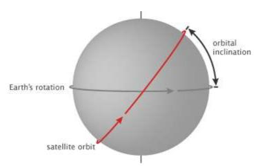
Orbital inclination is the angle between the plane of an orbit and the equator. An orbital inclination of 0° is directly above the equator, 90° crosses right above the pole, and 180° orbits above the equator in the opposite direction of Earth's spin. (NASA illustration by Robert Simmon.)
