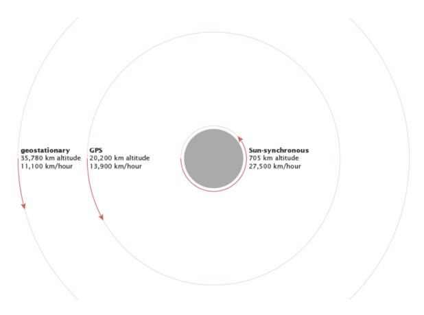
The higher a satellite's orbit, the slower it moves. Certain orbital altitudes have special properties, like a geosynchronous orbit, in which a satellite travels around the Earth exactly once each day. The length of each red arrow in this diagram represents the distance traveled by a satellite in an hour. View animation. (NASA illustration by Robert Simmon.)
