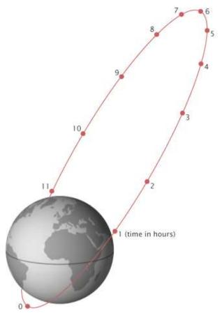
The Molniya orbit combines high inclination (63.4°) with high eccentricity (0.722) to maximize viewing time over high latitudes. Each orbit lasts 12 hours, so the slow, high-altitude portion of the orbit repeats over the same location every day and night. Russian communications satellites and the Sirius radio satellites currently use this type of orbit. (Adapted from *Fundamentals of Space Systems* by Vincent L. Pisacane, 2005.)
