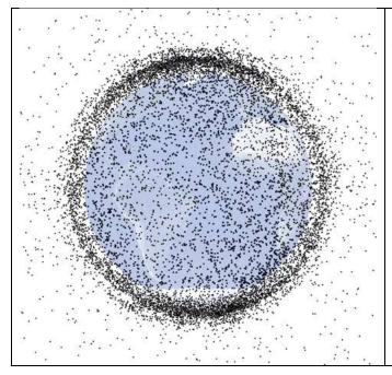
Thousands of manmade objects—95 % of them "space junk"— occupy low Earth orbit. Each black dot in this image shows either a functioning satellite, an inactive satellite, or a piece of debris. Although the space near Earth looks crowded, each dot is much larger than the satellite or debris it represents, and collisions are extremely rare. (NASA illustration courtesy Orbital Debris Program Office.)
