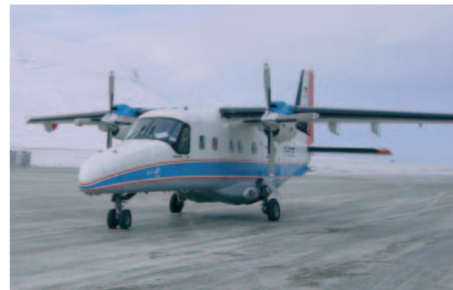
The AW1 Dornier 228 aircraft carrying the ESA radar altimeter ASIRAS along with a laser altimeter. This aircraft was used for 2004 pre-launch validation experiments focused mainly on land-ice validation
