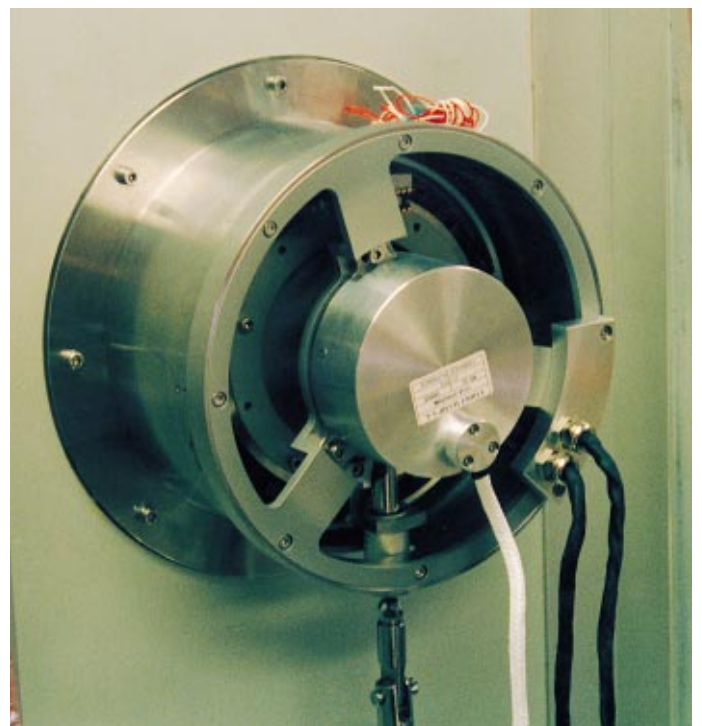
Figure 7. The scan mechanism, with the optical encoder in the foreground
