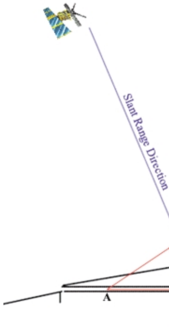
Figure 7. ERS SAR slant-range viewing with respect to the geological fault movement. A simple geometrical function can be used to determine the movements horizontal component.
