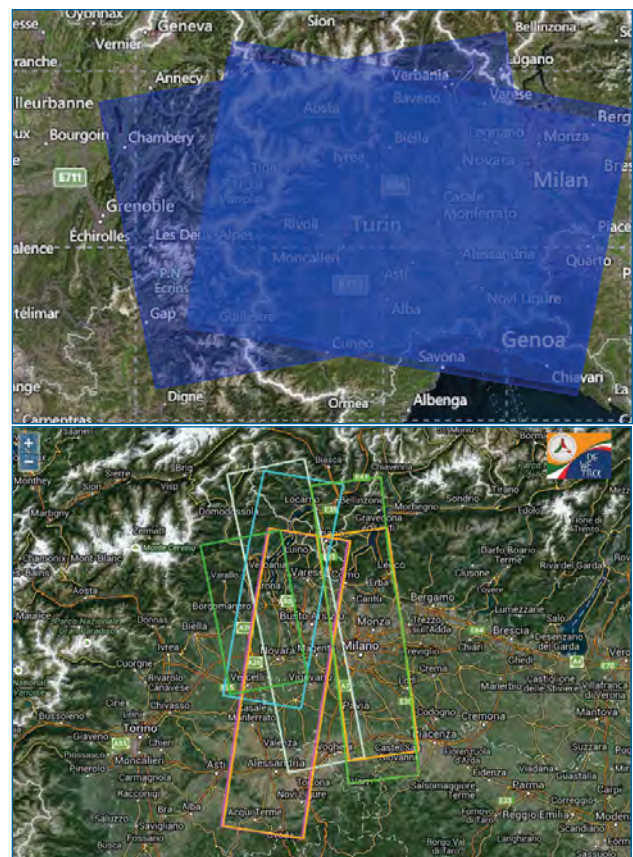
Figure 3: Spatial and temporal coverage of the AOI by Sentinel-1A (top) and CSK (bottom) for the period November 13–20, 2014.
