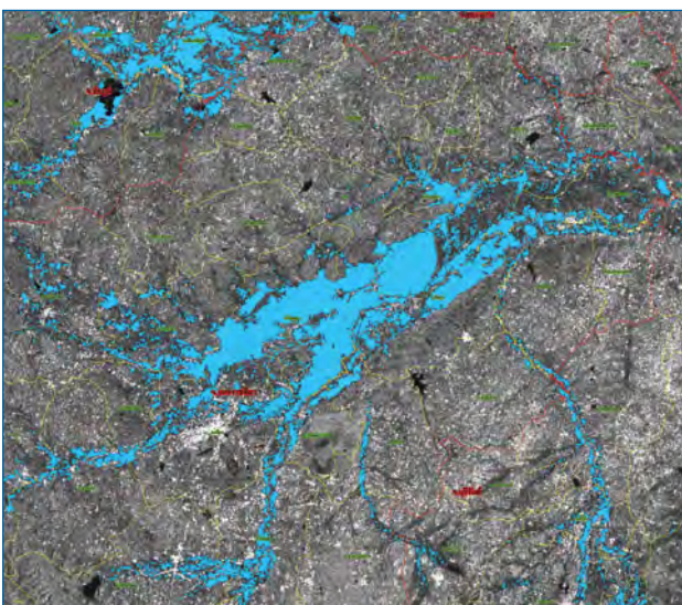
Figure 4: Flood inundation map generated using ALOS/PALSAR imagery. Blue shows the inundation area extracted from satellite imagery analysis.
