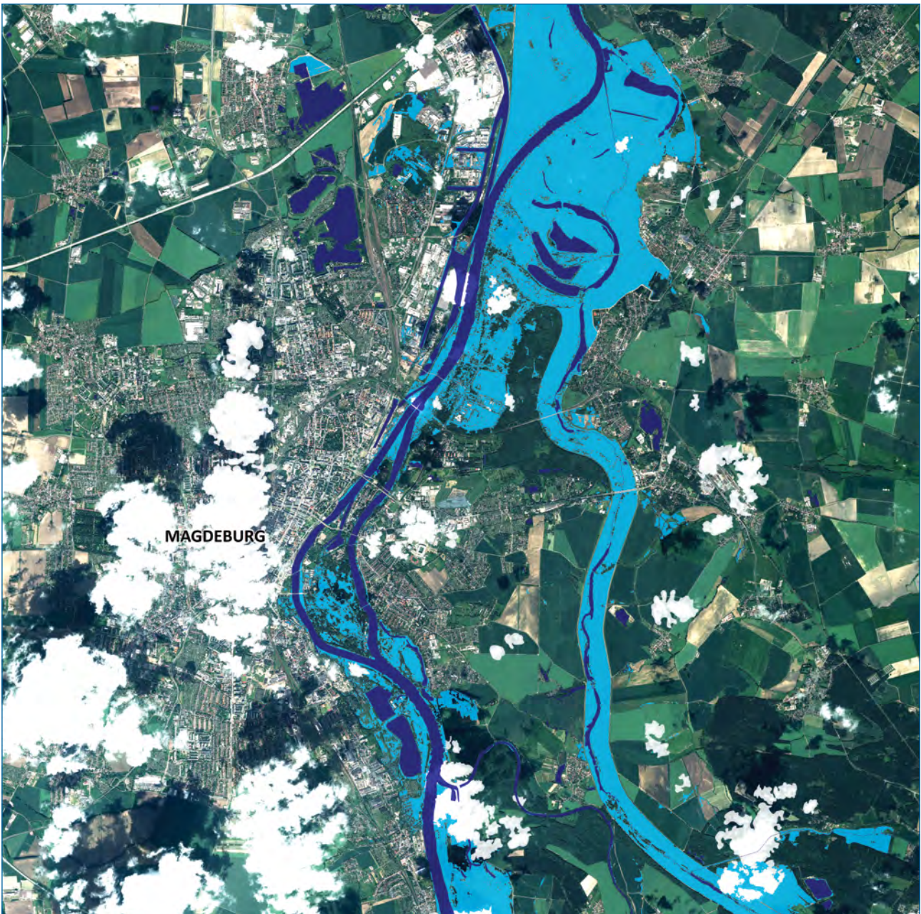
Figure 1: Rapid Flood Extent over the city of Magdeburg, Germany, derived from a Pléiades-HR data (70cm) acquired the 10th of June 2013 during the Elbe River flood event.
