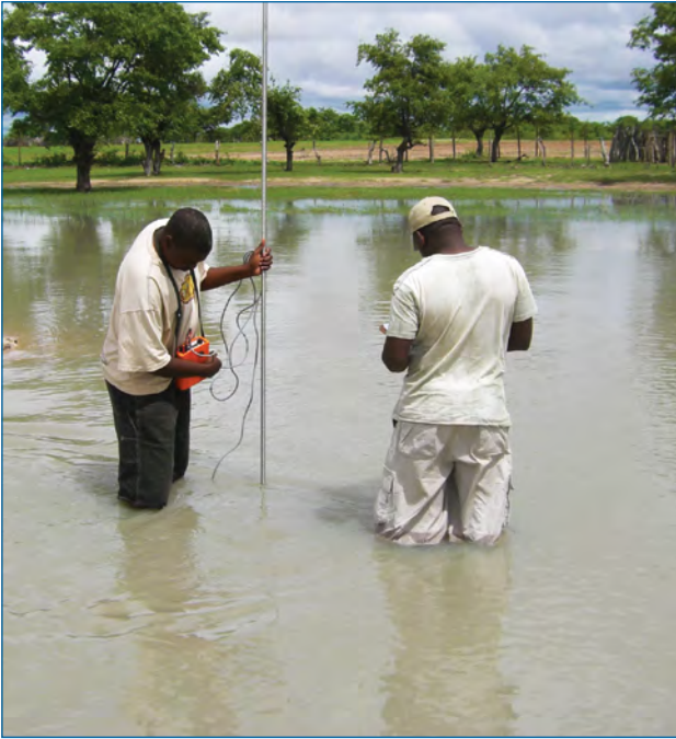
Figure 1: Namibian hydrologists manually measure flood water depth for map validation.
