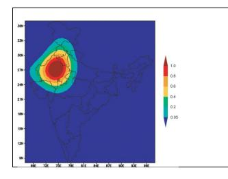
The averaging function (spatial weighting) used to estimate terrestrial water storage changes from GRACE data is mapped. Warmer colors indicate greater sensitivity to terrestrial water storage changes. Credit: NASA/Matt Rodell > Larger image
