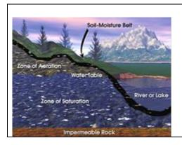
Groundwater resides beneath the soil surface in permeable rock, clay and sand as illustrated in this conceptual image. Many aquifers extend hundreds of feet underground and in some instances have filled with water over the course of thousands of years. **Credit:** NASA
