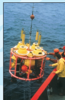
Bottom pressure sensing instrument MYRTLE, being deployed in the South Atlantic
