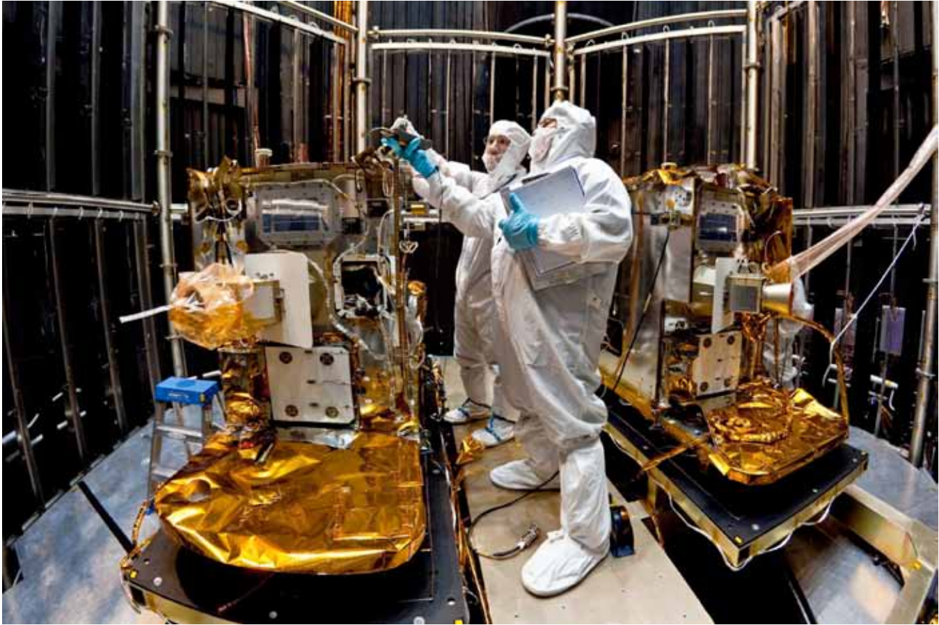
Technicians prepare to hoist one of the two GRAIL spacecraft upon completion of a thermal vacuum test at the Lockheed Martin Space Systems facility in Denver. Image Credit: NASA/JPL-Caltech/LMSS
