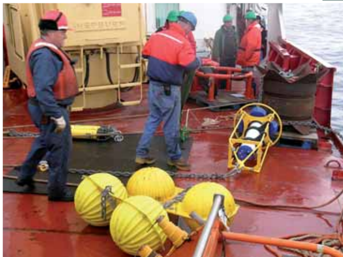
Preparing for deployment of a mooring with hardhats, an ADCP, acoustic releases and the bottom anchor. (Fiamma Straneo, Woods Hole Oceanographic Institution)
