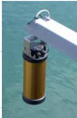
The Ott Radar Unit records sea level by acoustically measuring the distance from the transducer head to the water surface. (Proudman Oceanographic Laboratories)
